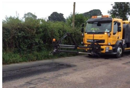
The 18-tonne machines fill and seal potholes remotely without refilling through the day - rather than send crews out to locations to carry out repairs. The 'pothole zappers' also create no waste, meaning they are more environmentally friendly than traditional filling methods.
